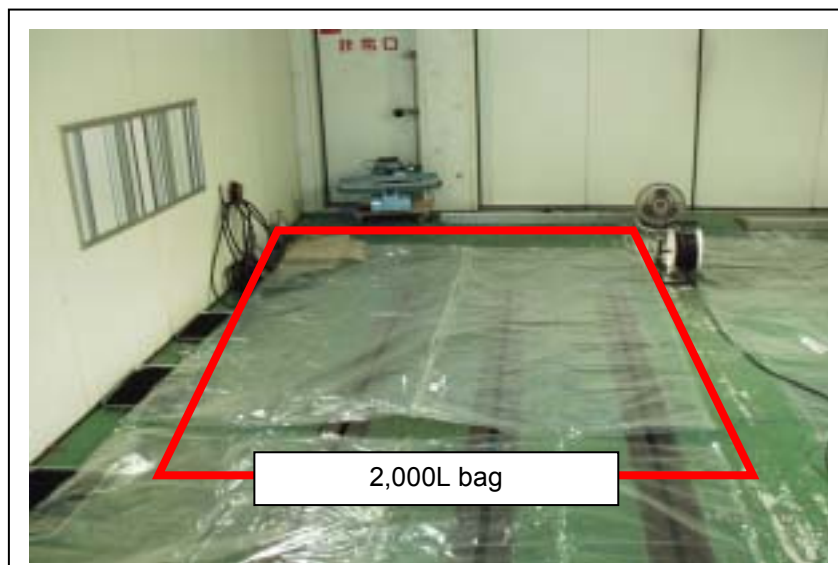
Figure 11. Condition in which the bag of 2,000L is prepared in the test chamber
