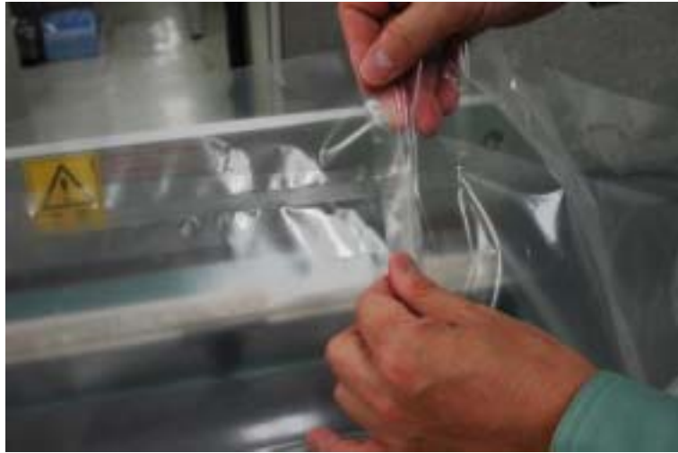
Figure 7. Welding is performed twice to prevent a leak.
