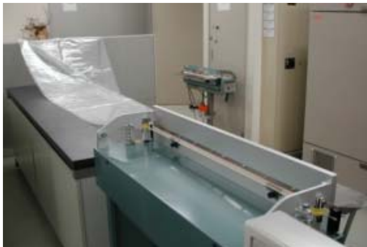
Figure 5. The side of 5m is welded using the sealer.
